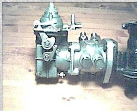
This photo shows the engine side of the metering unit, the full throttle screw can be seen on the bottom. The cold enrich screw is almost visible above and to the left of the full throttle screw. The lock nuts are exposed (black cover removed) in the upper left side of the metering unit. I have been able to adjust the cold enrich screw with a wrench but it's not easy!
